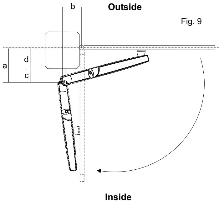
Total stroke 400 mm - max. recommended stroke 380 mm
