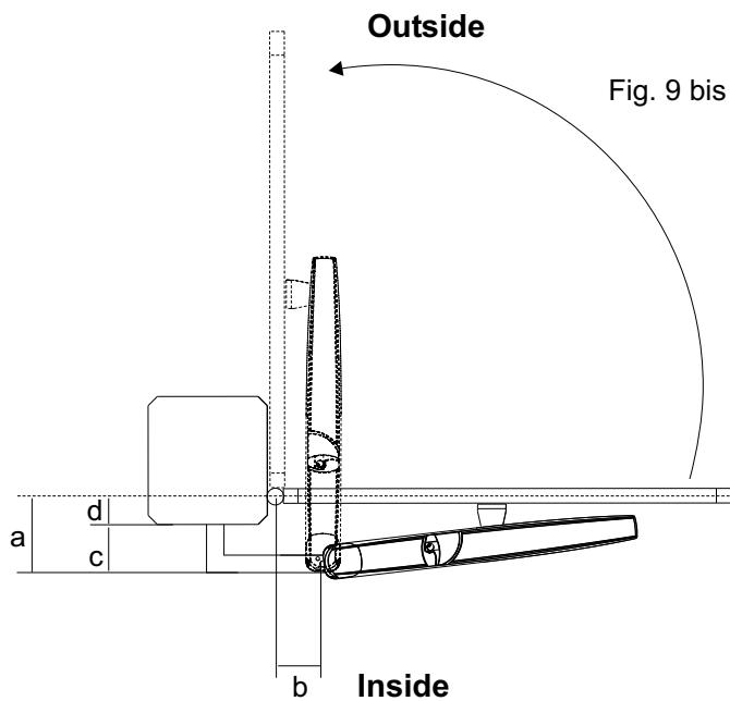
Total stroke 400 mm - max. recommended stroke 380 mm
