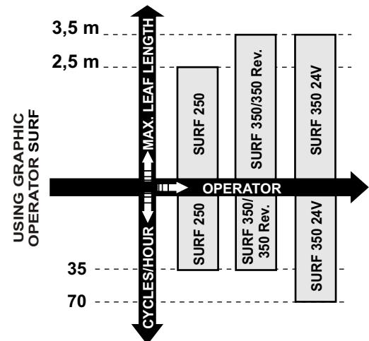
**Note:** The frequency of use is valid only for the first hour at 20°C room temperature.
