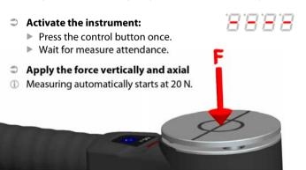
Within five seconds from of the 20N - trigger the force signal is evaluated according to EN12453 and DIN18650.
